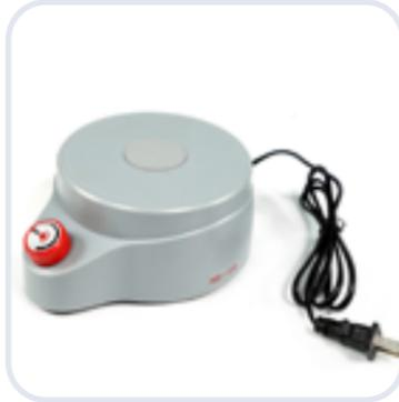
Magnetic stirrer is an instrument for liquid mixing, mainly used for liquid reagent configuration, stirring low viscosity liquid or solid-liquid mixture; MS-150 magnetic stirrer has a large stirring volume, stable rotor rotation, no jumping sub, and its shell is molded by flame retardant reinforced plastic as a whole, fully enclosed waterproof and rustproof.
