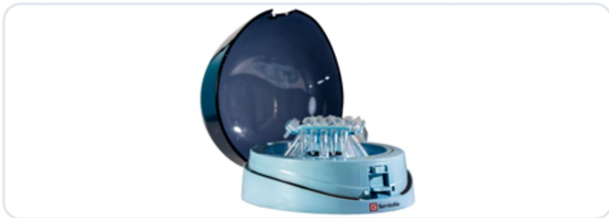
Servicebio mini centrifuges are widely used for the separation and purification of microscopic items, and also for mixing experiments. Applications: serum extraction from whole blood, supernatant extraction from various samples, rapid sample sedimentation, microscopic blood cell separation, microbial sample processing and PCR experimental partition centrifugation, etc.
