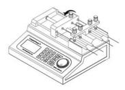
3 Turn the Drive Nut Knob according to the arrow head direction and make the drive nut engage the leadscrew. Then the pump is in the working state.
