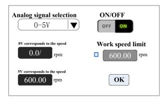
Click the **System Settings** button in the main interface, then click **External Speed Control** button to enter External Speed Control Settings interface.
