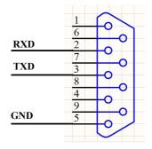
⑦ RS485 Communication Interface: Choose RS485 in the communication setting interface, this terminal is active.
