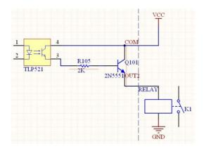
If connect with relays, when the motor runs, K1 connect; when the motor stop running, the K1 disconnect.
