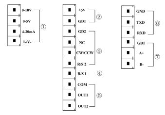
① Analog signal input terminal: Choose the External speed control signal and turn on the Ext. Speed in external control setting interface, control the motor speed from 0 rpm to maximum speed through analog signal.
