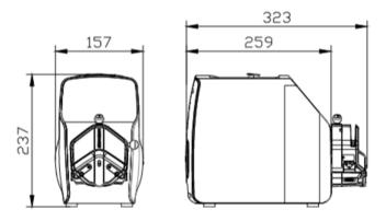
LabV+EasyPump pump head
