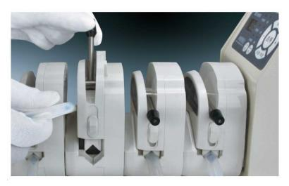
Mounting several pump heads can increase the flow rates
